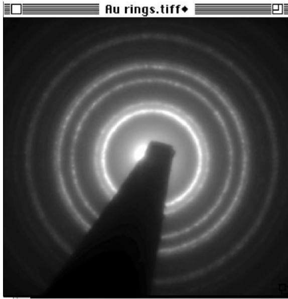
Figure 3.2. Electron diffraction pattern obtained by hitting Au atoms with a beam of electrons. Courtesy of Eric Steel, National Institute of Standards and Technology (NIST).
